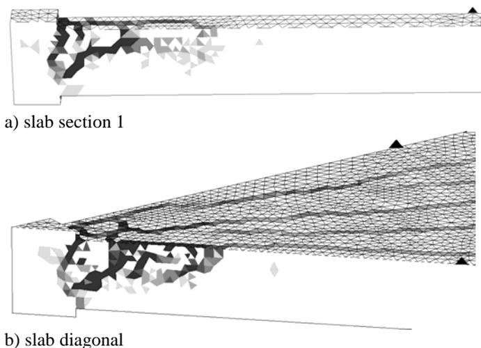
Figure 9. Cracking at ultimate load: SB1.
