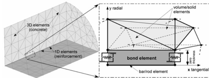
Figure 4. Definition of the bond element.
