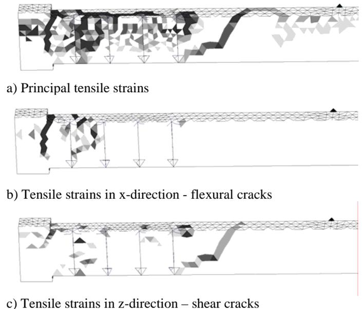
Figure 10. Cracking at ultimate load: SB4 section 1.
