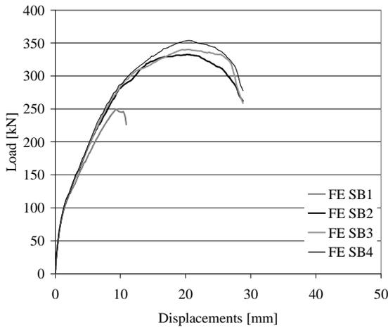
Figure 8. Load displacement curves simulations.
