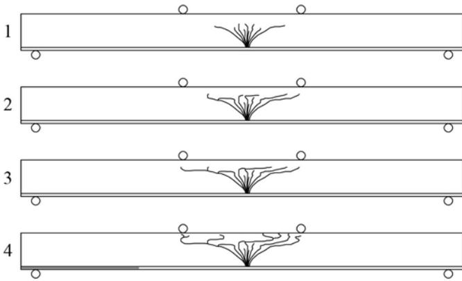
Figure 11. Schematic overview of crack propagation, at different time steps (1-4), for L II – GB368 specimens.
