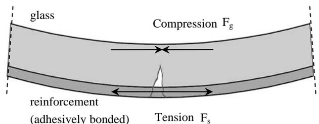
Figure 1. Reinforced glass beam concept: schematic overview of distribution of forces after glass failure.
