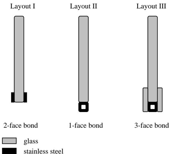
Figure 2. Tested reinforcement layouts.
