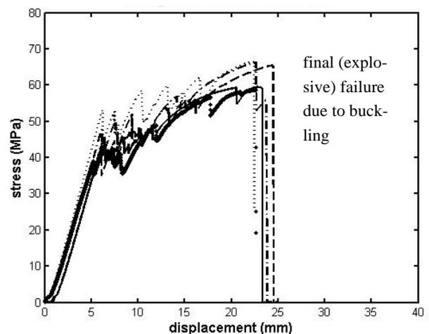
Figure 14. Stress-displacement diagram of layout III - AR2013 specimens.
