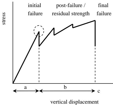
Figure 4. Schematic stress-displacement diagram for all reinforcement layouts.
