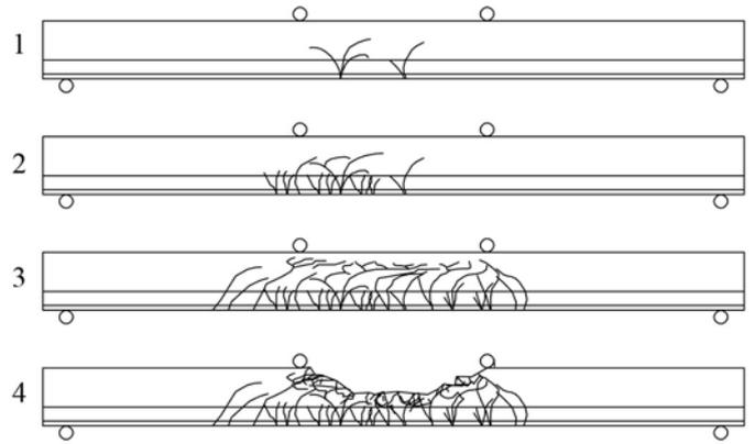
Figure 17. Schematic overview of crack propagation, at different time steps (1-4), for L III – AR2013 specimens.
