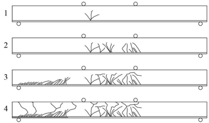
Figure 12. Schematic overview of crack propagation, at different time steps (1-4), for L II – AR2013 specimens.
