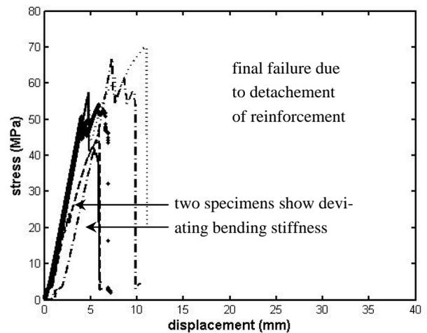
Figure 9. Stress-displacement diagram of layout II - GB368 specimens.
