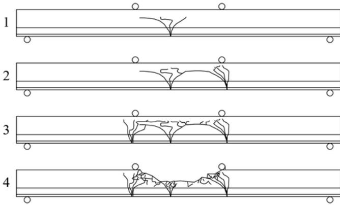
Figure 15. Schematic overview of crack propagation, at different time steps (1-4), for L III – GB368 specimens.
