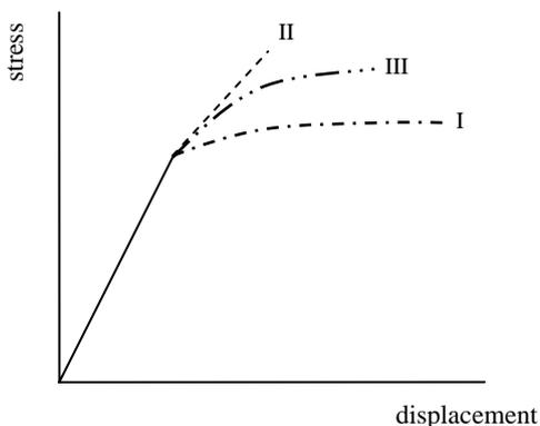
Figure 16. Schematic stress-displacement diagram of layout I, II and III.
