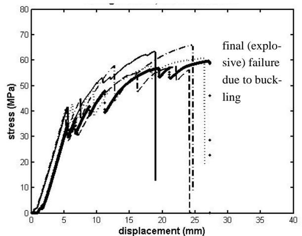
Figure 13. Stress-displacement diagram of layout III - GB368 specimens.
