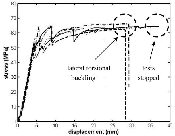
Figure 5. Stress-displacement diagram of layout I - GB368 specimens.
