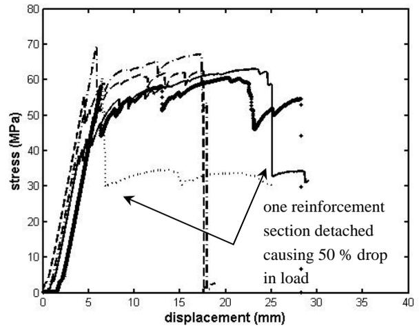
Figure 6. Stress-displacement diagrams of layout I - AR2013 specimens.
