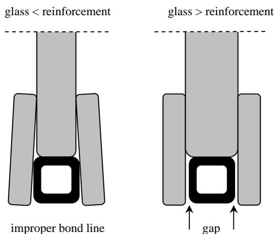
Figure 3. Effects of dimensional inaccuracies for layout III.
