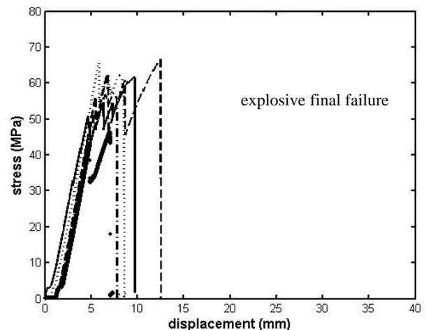
Figure 10. Stress-displacement diagram of layout II - AR2013 specimens.
