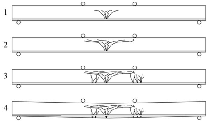
Figure 8. Schematic overview of crack propagation, at different time steps (1-4), for L I – AR2013 specimens.
