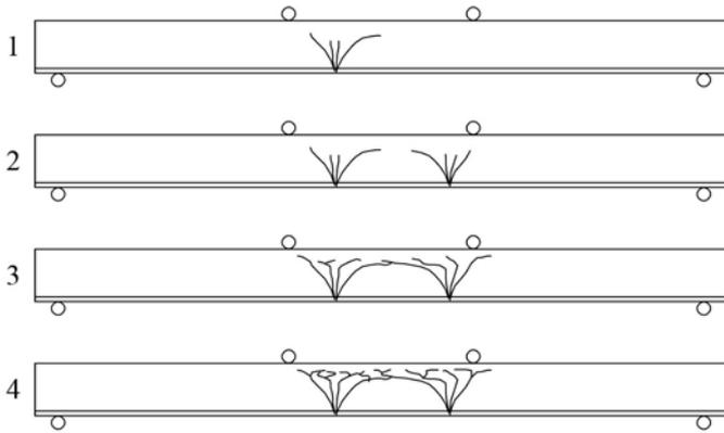
Figure 7. Schematic overview of crack propagation, at different time steps (1-4), for L I – GB368 specimens.
