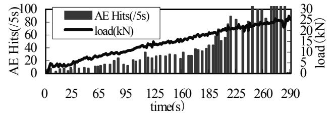
Figure 3 AE generation behaviors in the compression test (fracture position).
