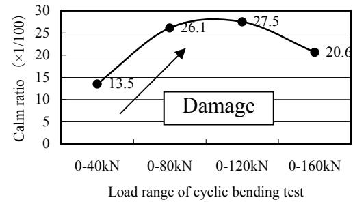
Figure 9 Calm ratios in the cyclic bending test.
