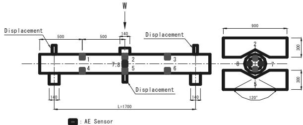
Figure 2 AE sensor arrangements in the bending test.
