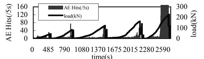
Figure 6 AE generation behaviors in the cyclic bending test.
