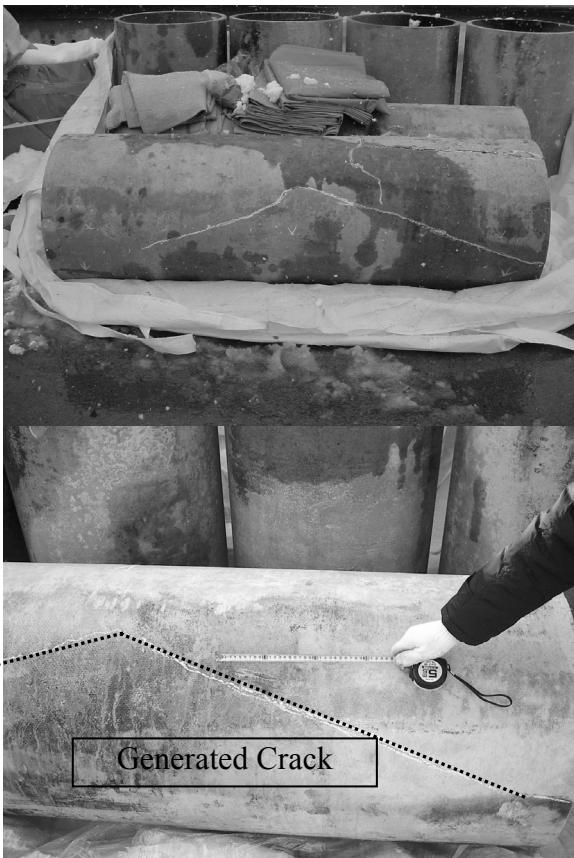
Figure 8 Result of Fracture in bending test.
