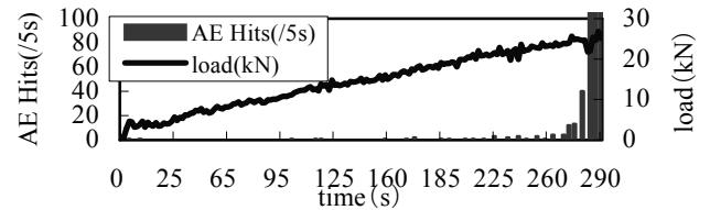
Figure 4 AE generation behaviors in the compression test (sound position).
