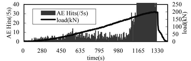
Figure 5 AE generation behaviors in the bending test.
