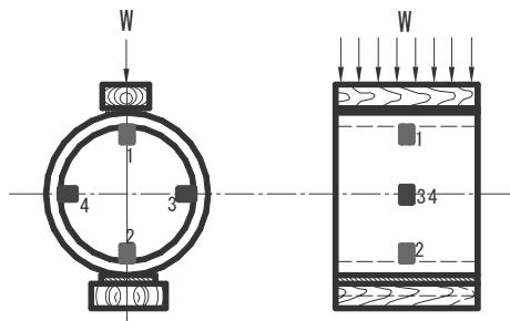
Figure 1 AE sensor arrangements in the compression test.
