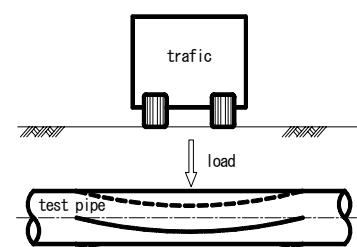
Figure 7 Loaded condition of a tested pipe.
