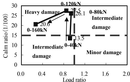
Figure 11 Relationships between the calm ratio and the load ratio.
