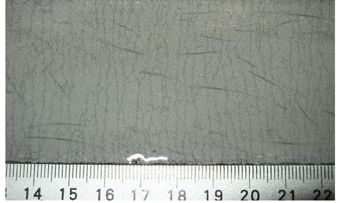
Figure 2. Distinctive fine multiple cracking upon strain hardening of UHP-FRC with only 1.5 % twisted high strength steel fibers.
