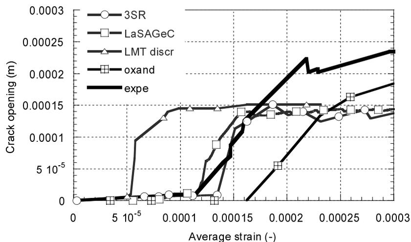
Figure 9. Opening of the second crack as a function of the average strain.
