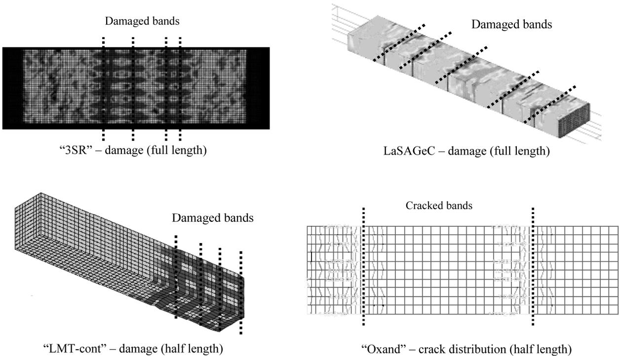
Figure 6. Characterization of the mechanical degradation (average strain = 0.3 0/00).
