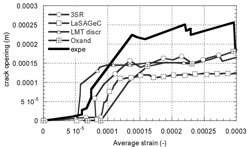
Figure 8. Opening of the first crack as a function of the average strain.
