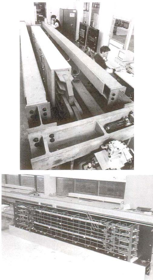
Figure 1. Experimental device for reinforced concrete ties (Mivelaz, 1996).
