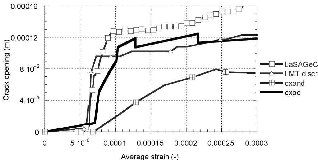
Figure 11. Evolution of the crack opening as a function of the average strain (case R5).
