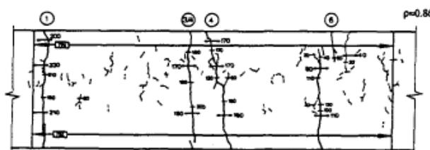
Figure 7. Experimental crack distribution (Mivelaz, 1996).
