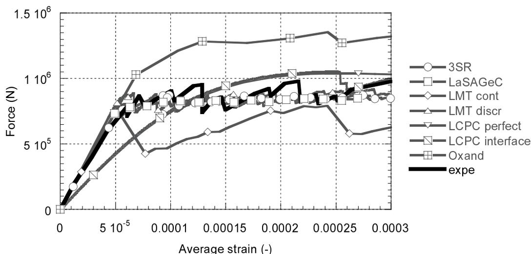
Figure 10. Evolution of the force as a function of the average strain (case R5). Zoom on the first part of the loading.
