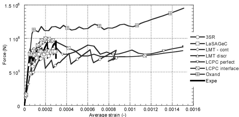
Figure 4. Force as a function of the average strain. Evolution on the total loading.
