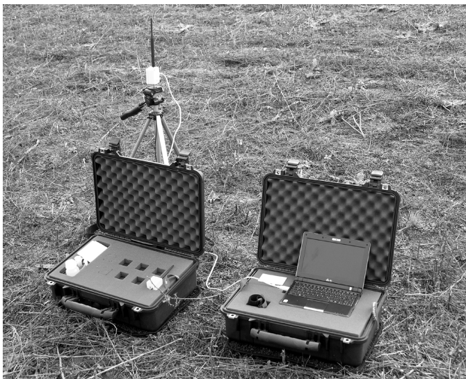
Figure 8. Measuring system consisting of the receiver box on a tripod, a mobile computer and the transport cases.
