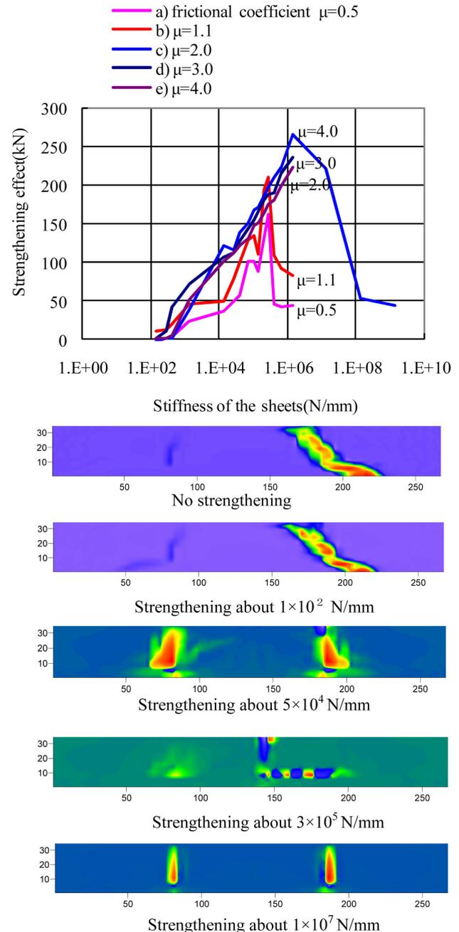
Figure 7. Shift in strain distribution at softening zone by increasing strengthening stiffness.
