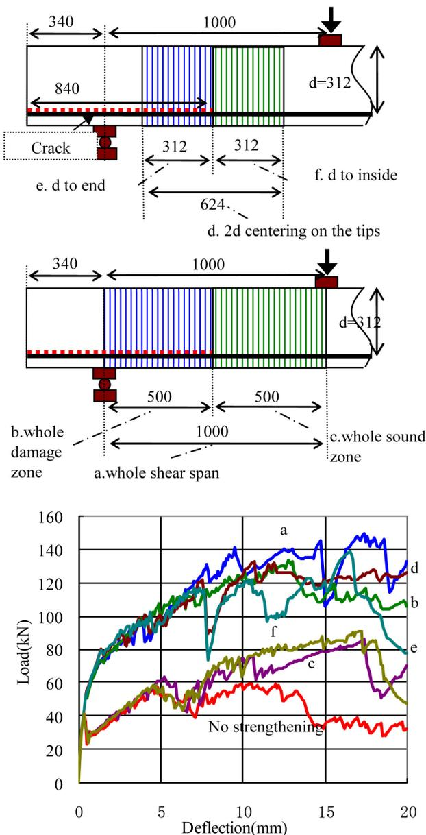
Figure 8. Analytical cases of the different strengthening and comparison of their strengthening effects.
