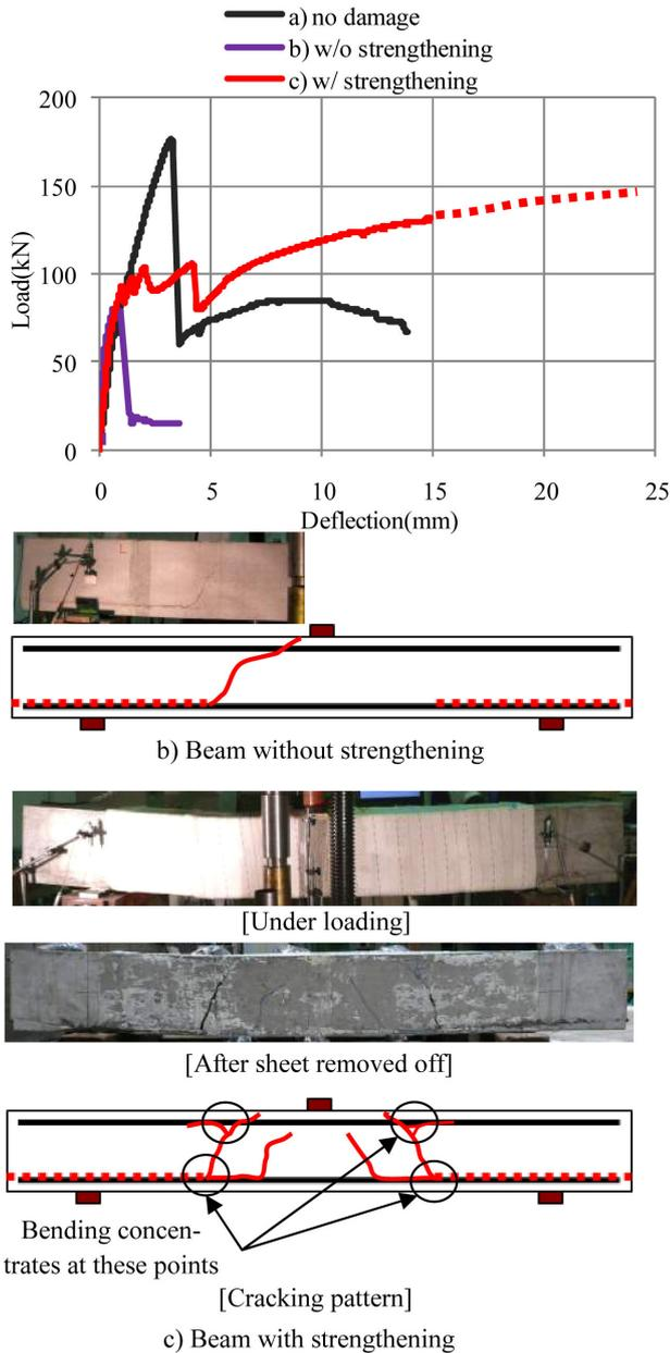
Figure 3. Comparison of the loading test results between without and with strengthened beams.
