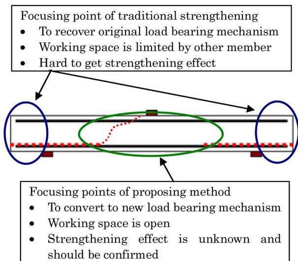
Figure 2. Concept of strengthening damage expected.
