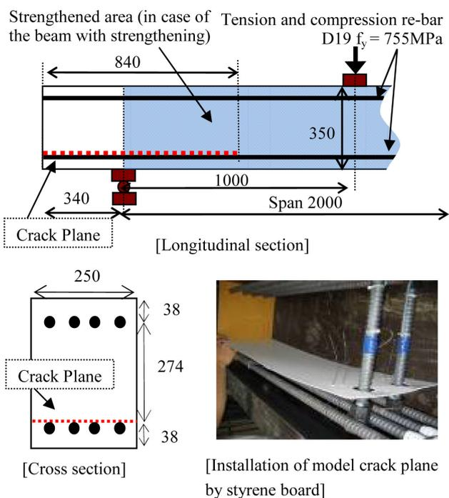
Figure 1. Detail design of the target beam.
