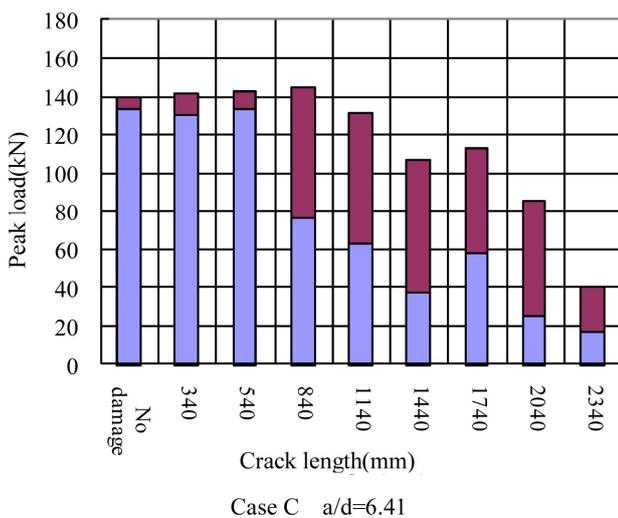
Figure 10. Shifting strengthening effect depending on the crack extending from the end of the beam.
