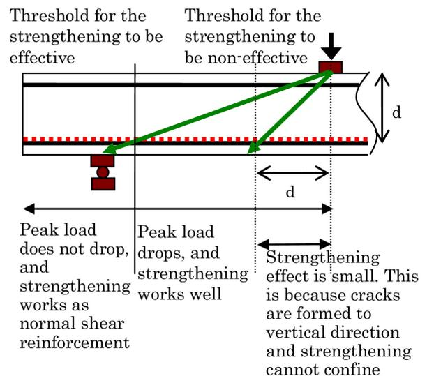
Figure 11. Classification of the strengthening mechanism.
