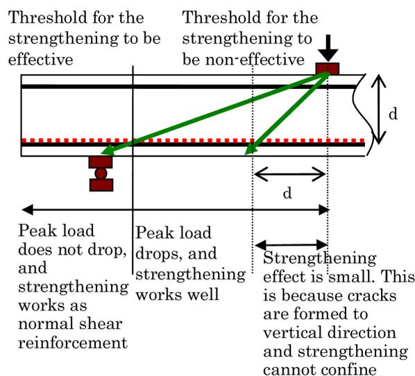
Figure 11. Classification of the strengthening mechanism.
