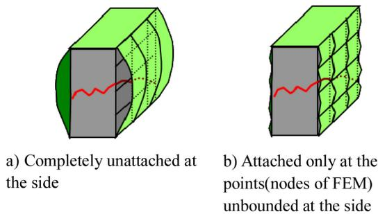
Figure 5. Bond between sheet and concrete in analysis.
