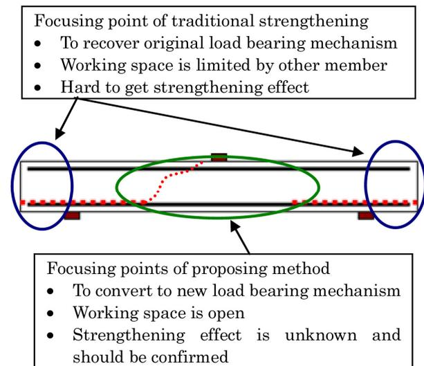
Figure 2. Concept of strengthening damage expected.
