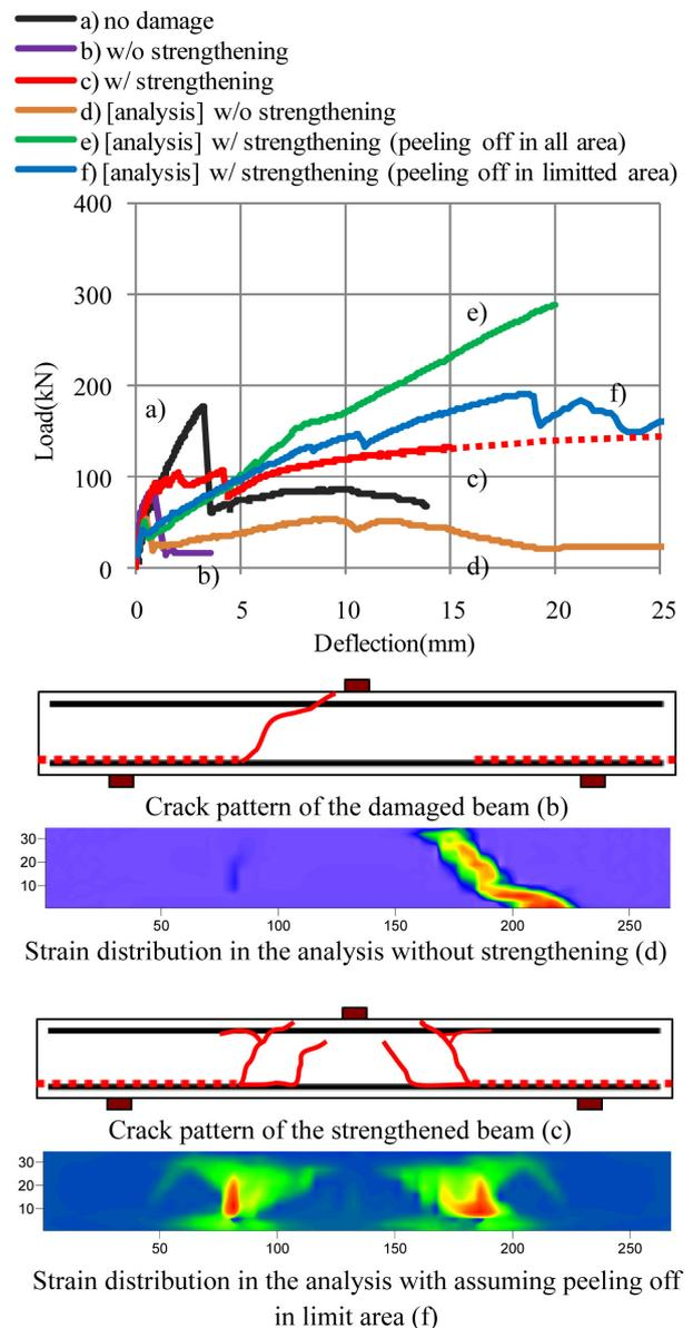
Figure 6. Comparison of analytical results of the beams with and without strengthening.
