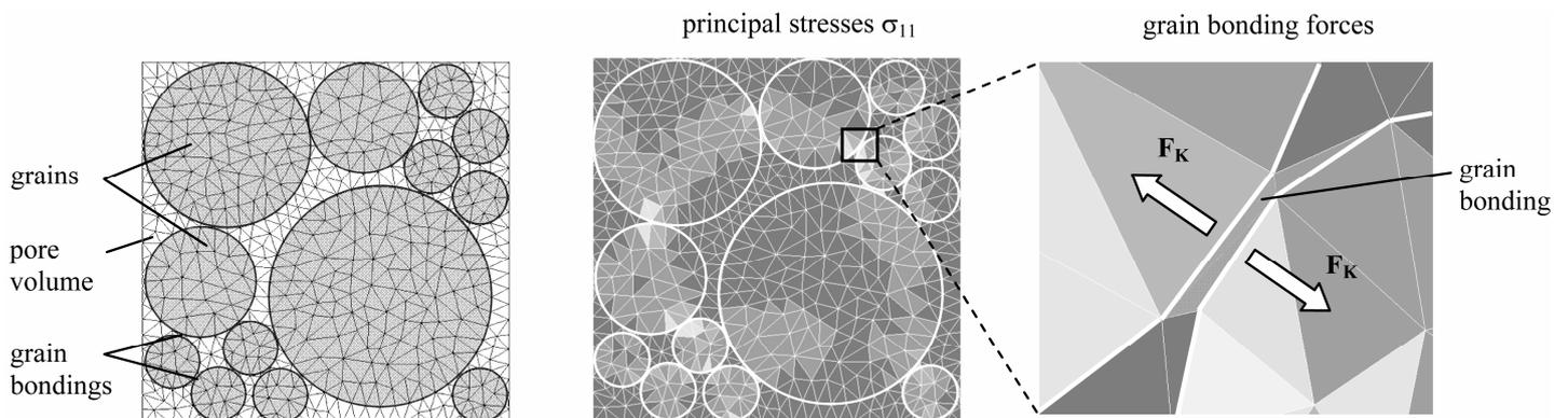
Figure 10. Randomly generated structural model depending on porosity and grain size distribution of the real sandstone (left) and exemplary presentation of computation results of grain bonding forces (right).
