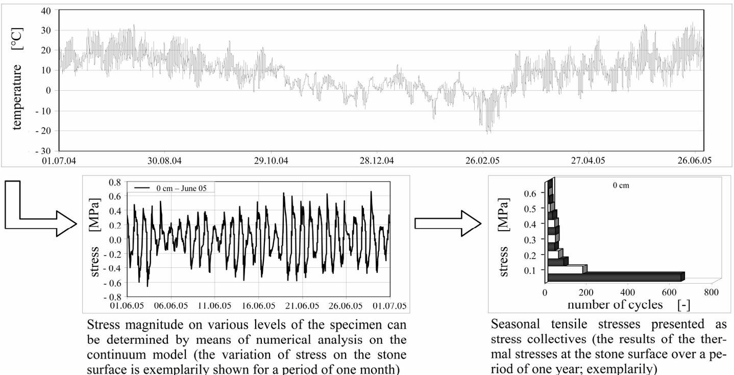
Figure 8. Presentation of exemplary test results on the continuum model.
