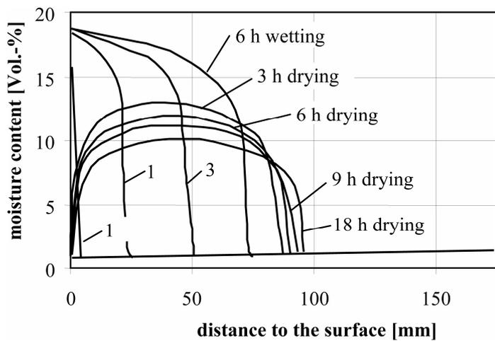
Figure 5. Moisture distribution in the stone – 6 hours of wetting followed by 18 hours of drying.
