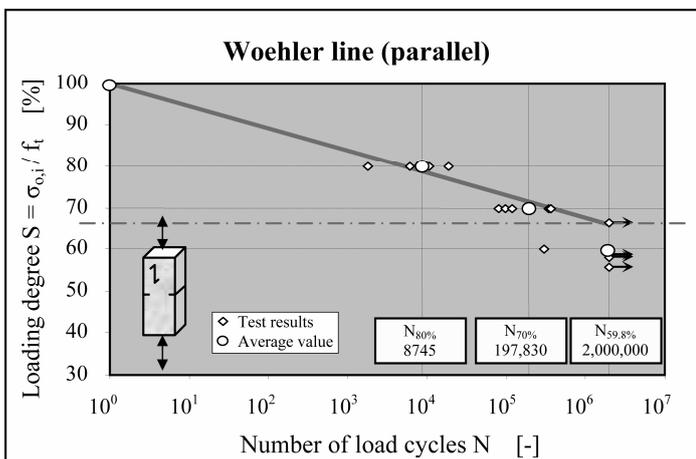
Figure 3. Test results of the dynamic tensile tests.
