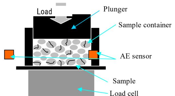
Figure 1. Sketch of aggregate loading test.
