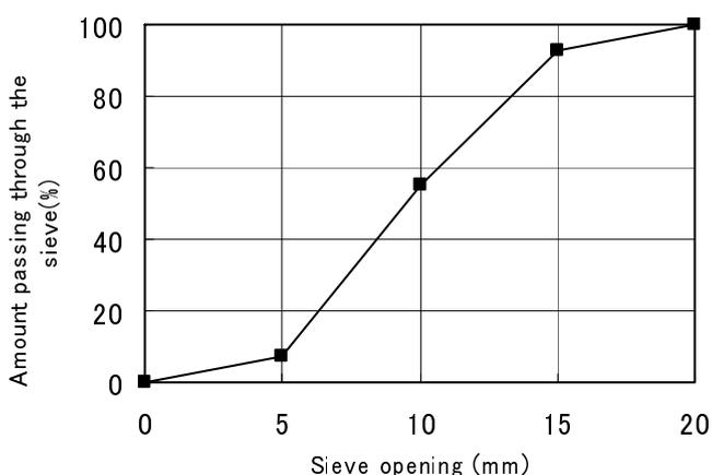
Figure 3. aregate gradation curve.
