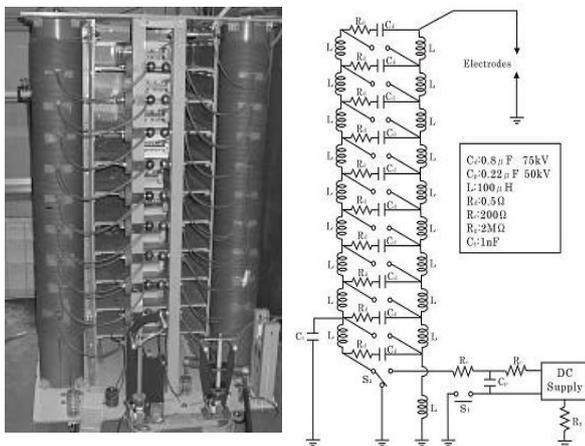
Figure 3. Marx Generator and its circuit.
