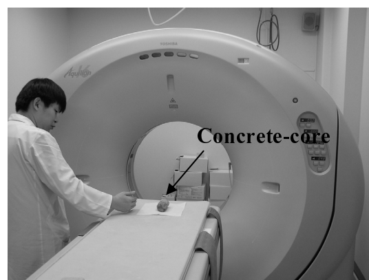
Figure 7. A general view of CT machine during concrete core scanning.
