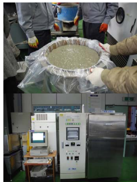
Figure 1. Test process for adiabatic temperature rise of concrete.
