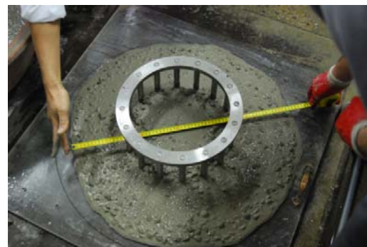
Figure 3. J-Ring test of fresh concrete.
