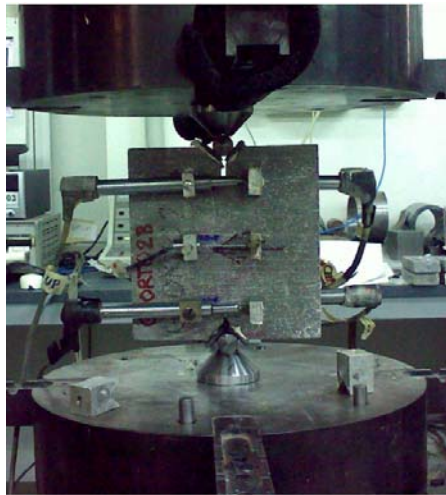
Figure 5. schematic of test set-up for DEWS tests (a) and picture of a specimen under testing (b).
