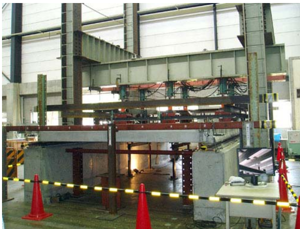
Photograph 8. Full scale loading experiment of UFC slab.
