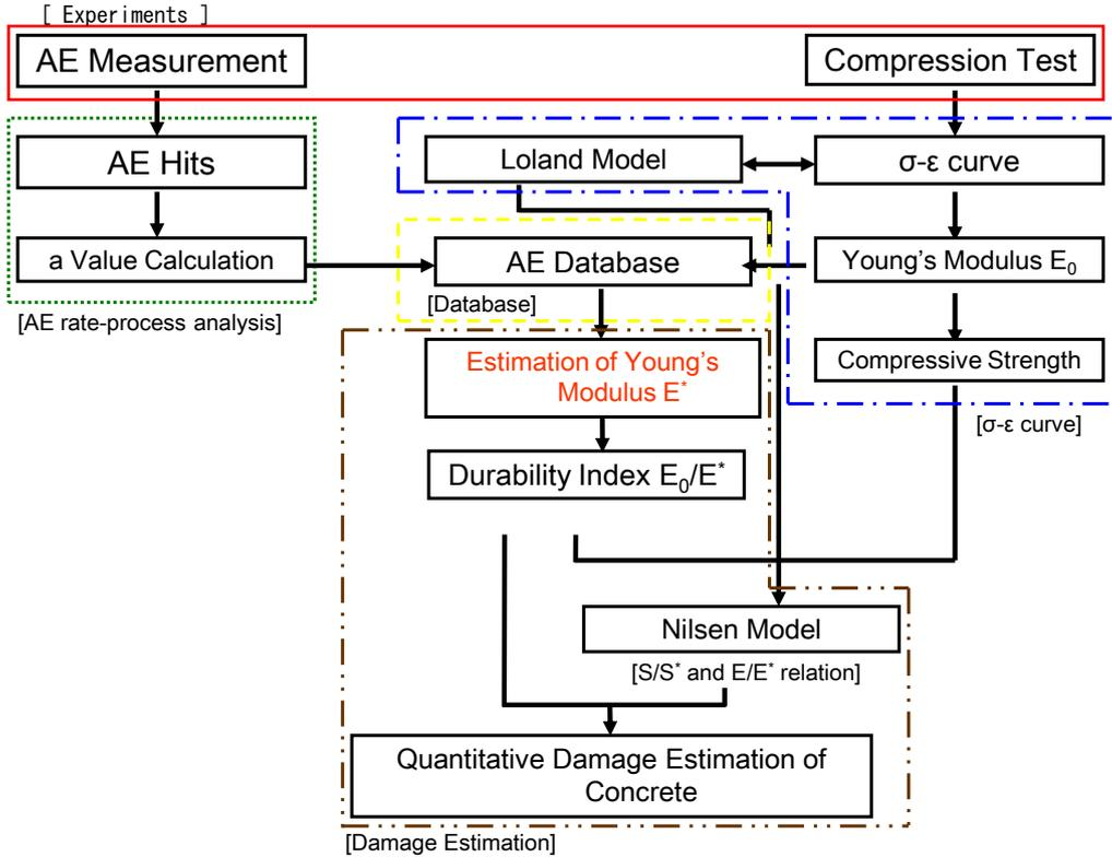
**Figure 1:** Analytical flow of DeCAT system.
