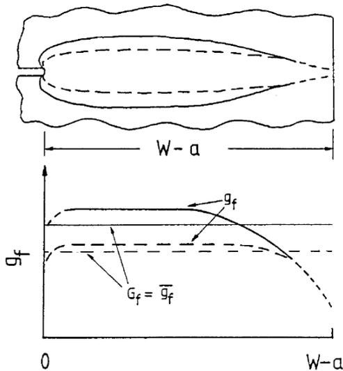
**Figure 1:** The local fracture energy  $g_f$  is constant if away from both front and back boundaries. The averaged  $G_f$  is specimen-size dependent.
