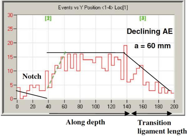
**Figure 2:** A tri-linear local fracture energy  $g_f$  can be assumed, as suggested by the AE measurements [30].
