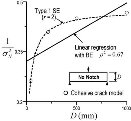
**Figure 5:** Predictions of Bazant’s SE model and FCM based on constant  $G_f$  for un-notched specimens, and  $\alpha_0 = 0.15$  was selected for BE model [12].
