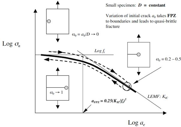
**Figure 4:** Interactions between FPZ and specimen boundaries for different crack/size ratios,  $\alpha_0 = a_0/D \rightarrow 0$  is the same as  $\alpha_0 \rightarrow 1$ .
