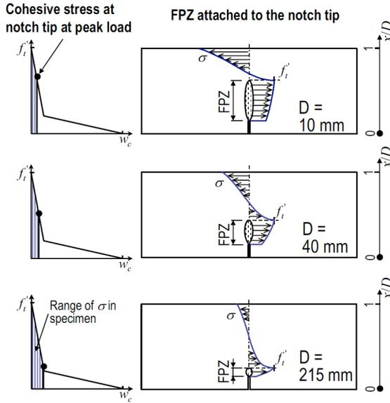
**Figure 3:** Simulated FPZ in different concrete specimens, using single tensile softening relation [12], while AE measurements suggest otherwise [26,27,30].
