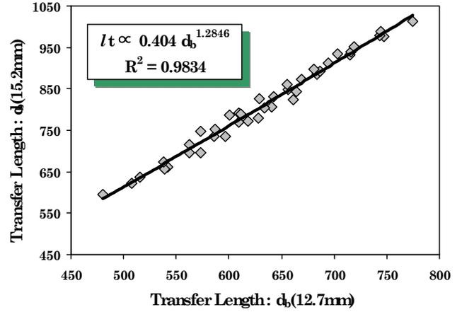
Figure 7: Variation of transfer length with strand diameter
