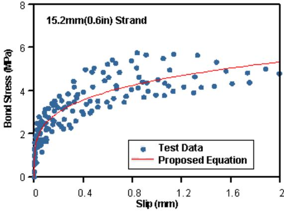
Figure 2: Bond stress and slip relation for strand
