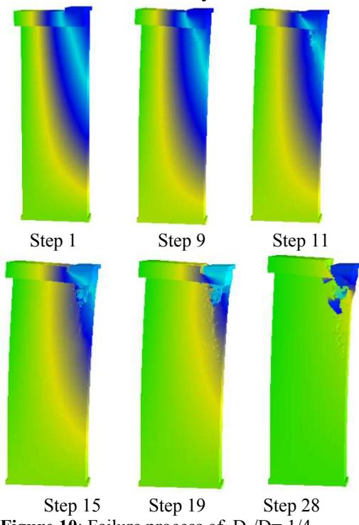
**Figure 10:** Failure process of  $D_1/D = 1/4$ .
