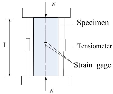
Figure 2 Schematic diagram of the compress experiment
