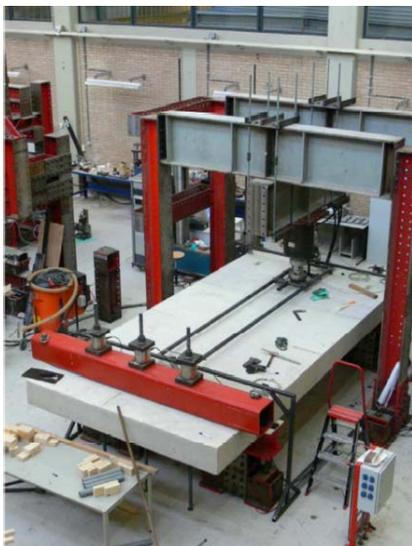
**Figure 2:** Experimental set-up of S1T1 slab.
