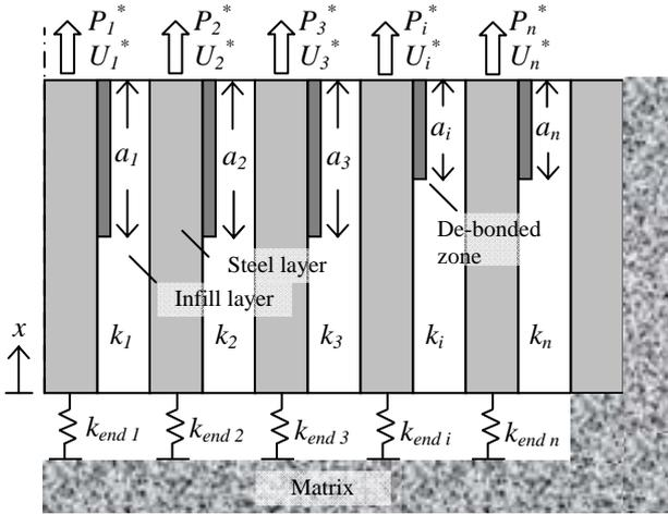
Figure 1: Multi-layer anchor-infill assembly.
