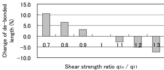
Figure 3: Influence of shear strength of infill material on de-bonded length.
