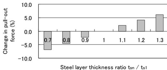
Figure 8: Influence of steel layer thickness on pull-out force.
