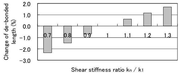
Figure 5: Influence of shear stiffness of infill material on de-bonded length.
