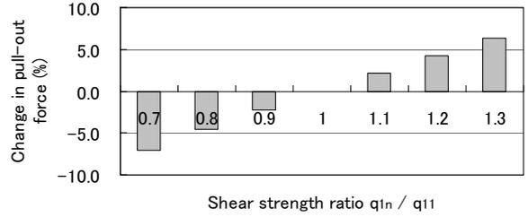
Figure 4: Influence of shear strength of infill material on pull-out force.
