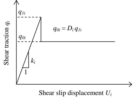
Figure 2: Mechanical behavior of infill material.
