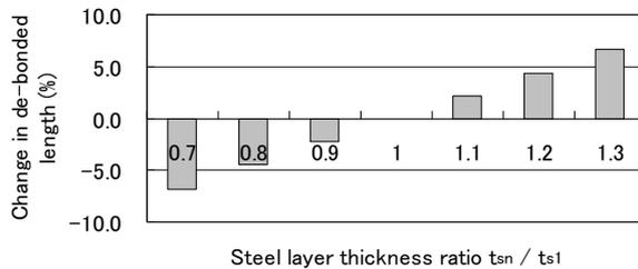
Figure 7: Influence of steel layer thickness on de-bonded length.
