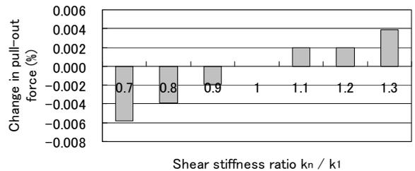
Figure 6: Influence of shear stiffness of infill material on pull-out force.
