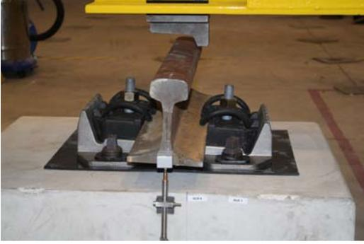
Figure 2: The cross-section profile of the UIC60 rail-fastening device seen within the experimental setup to measure its stiffness.
