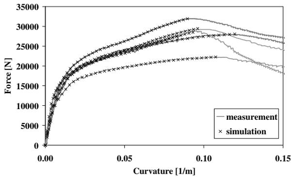
**Figure 12:** Comparison of measured and simulated force-curvature curves for the steel fibre reinforced mortar.
