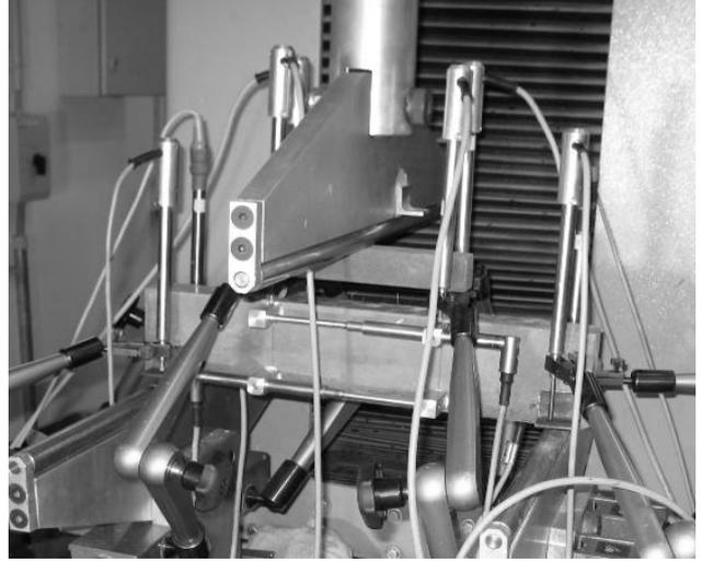
Figure 2: Experimental setup for the bending tests.
