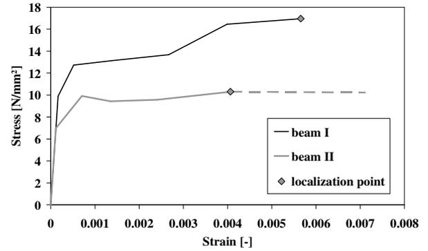
**Figure 17:** Obtained hardening curves for the steel fibre reinforced mortar.
