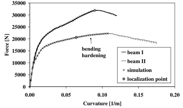
**Figure 16:** Comparison of measured and simulated force-curvature curves for the steel fibre reinforced mortar.
