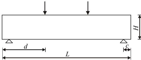
Figure 1: Geometry of the tested beams.
