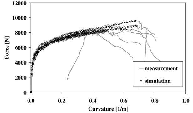
**Figure 10:** Comparison of measured and simulated force-curvature curves for the SHCC.
