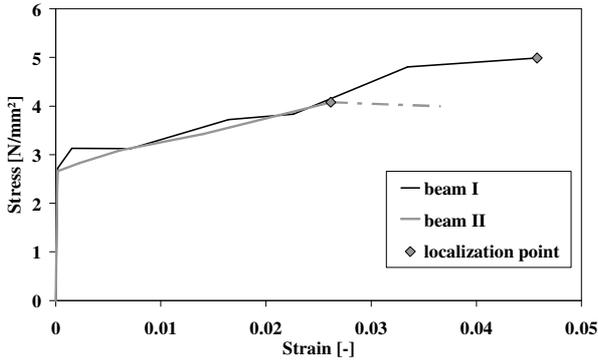
**Figure 15:** Obtained hardening curves for the SHCC.
