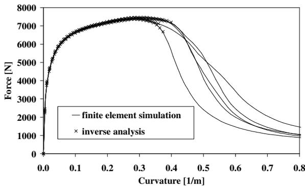
**Figure 7:** Simulation results of four-point bending tests.
