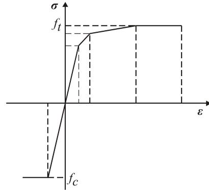
Figure 5: Stress-strain curve assumed for the nonlinear axial members.
