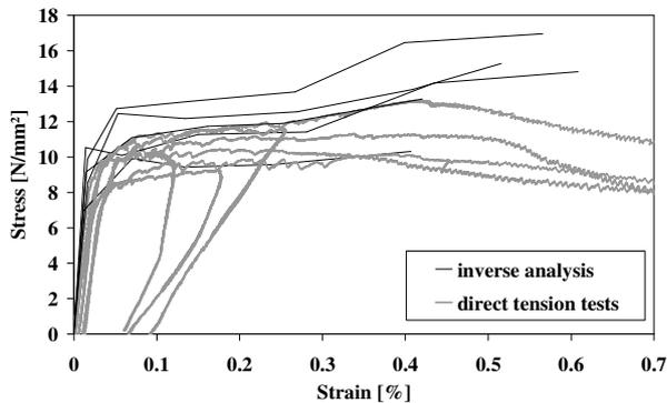
**Figure 13:** Obtained hardening curves for the steel fibre reinforced mortar.
