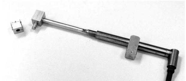
Figure 3: LVDT with hinge connectors for the curvature measurement.
