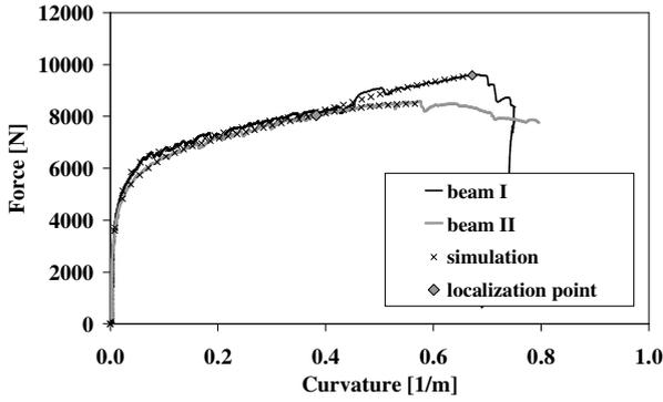
**Figure 14:** Comparison of measured and simulated force-curvature curves for the SHCC.
