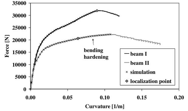
**Figure 16:** Comparison of measured and simulated force-curvature curves for the steel fibre reinforced mortar.
