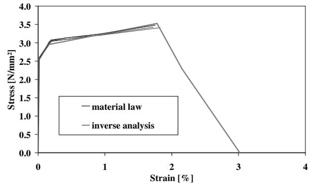
**Figure 9:** Hardening curves obtained by inverse analysis of the simulated four-point bending tests in comparison to the original material law.
