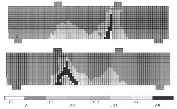
**Figure 8:** Simulation results of four-point bending tests, contours correspond to maximum principal strain.
