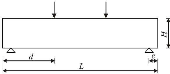
Figure 1: Geometry of the tested beams.
