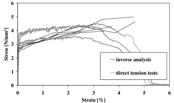
**Figure 11:** Obtained hardening curves for the SHCC.
