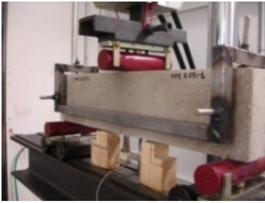
Figure 1: Three-point-bending test on single edge notched beams.
