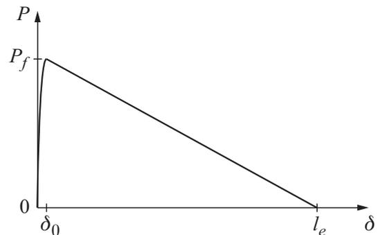
Figure 2: Pull-out load versus slip displacement for a fiber.
