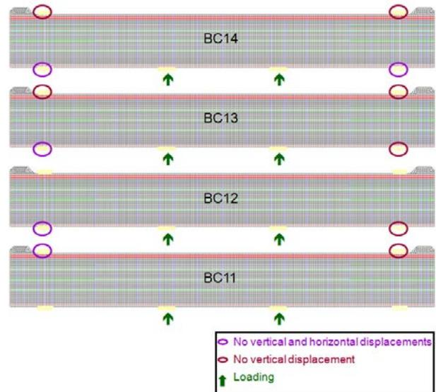
**Figure 7:** Boundary conditions for the first modelling.
