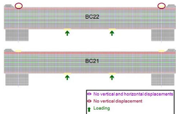
**Figure 8:** Boundary conditions for the second modelling.
