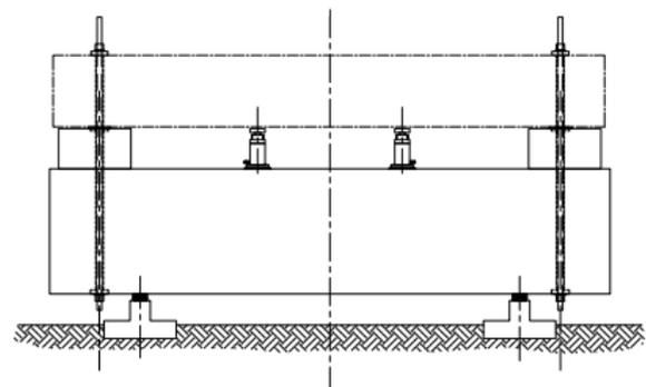
Figure 3: Loading setup of the beam.
