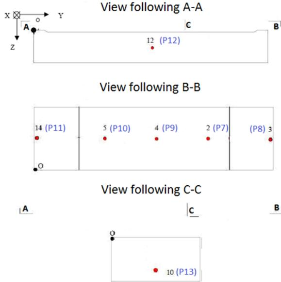
Figure 9: Position of the displacement sensors.
