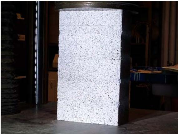
**Figure 1:** Stochastic patterns sprayed on a masonry prism surface.
