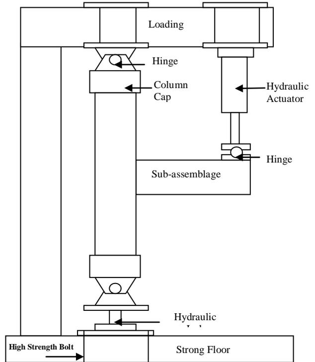
Figure 8: Diagram of the Experimental Set-up.
