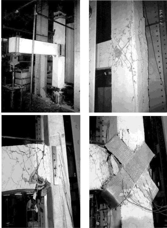
**Figure 3:** Joint failure of GRP rehabilitation
