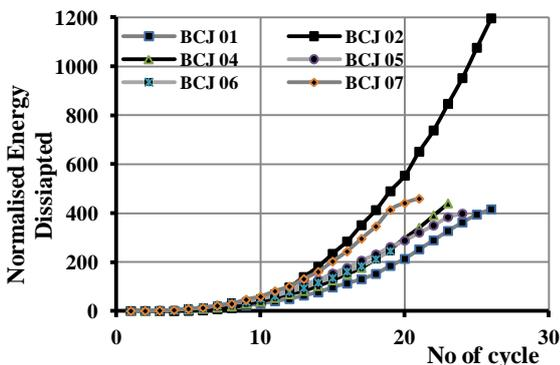
Figure 13: Cumulative Energy Dissipation.
