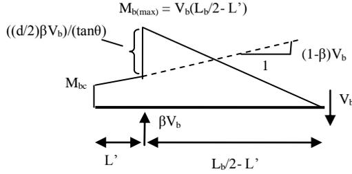
Figure 6a: BMD in beams with haunch elements.
