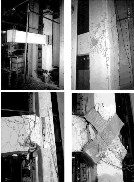
**Figure 3:** Joint failure of GRP rehabilitation
