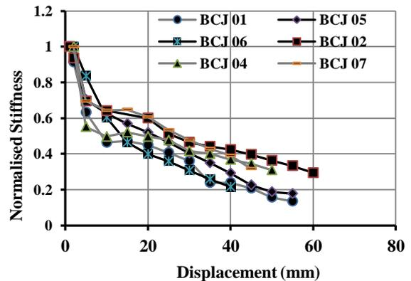
Figure 14: Stiffness Degradation in Sub-assemblies.
