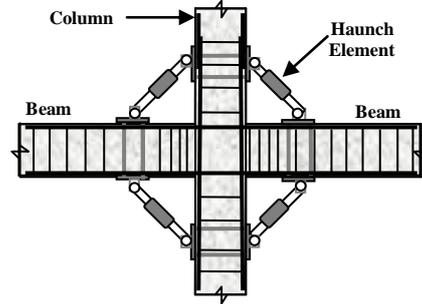
Figure 4b: Haunch retrofit scheme for interior joints.
