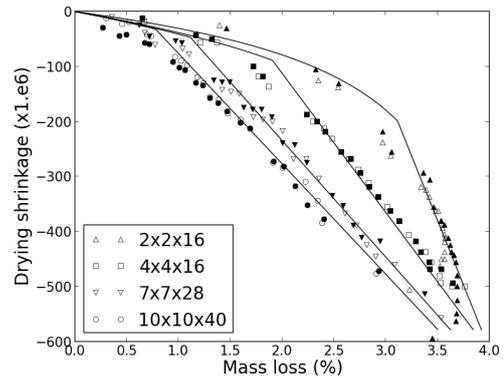
Figure 8: Prediction of the scale effect. Parameters are identified on the  $4 \times 4 \times 16$  cm sample.
