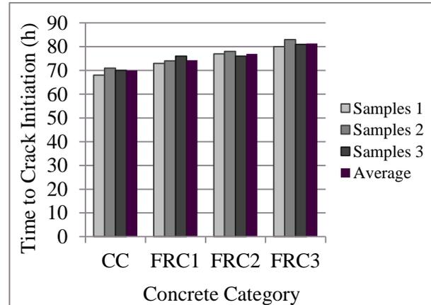
Figure 4: Time to cracking for different categories of concrete
