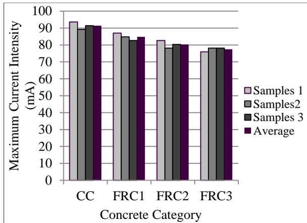
**Figure 5:** Maximum anodic current for different concrete categories utilizing impressed voltage technique
