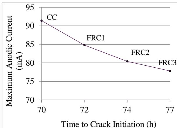
**Figure 6:** The average maximum anodic current versus the average time to crack initiation for concrete categories
