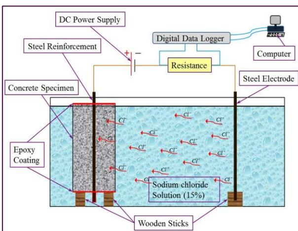
**Figure 1:** Accelerated Chloride-Induced Corrosion Test Set up
