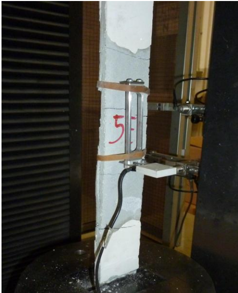
Figure 6: Cracking of the FRCM specimen with steel fibres.
