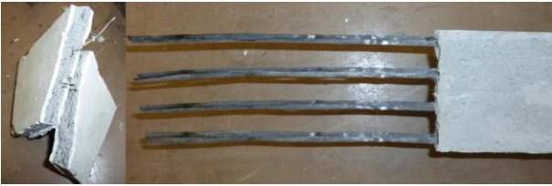
Figure 5: Extraction of the carbon fibre from the cementitious matrix.
