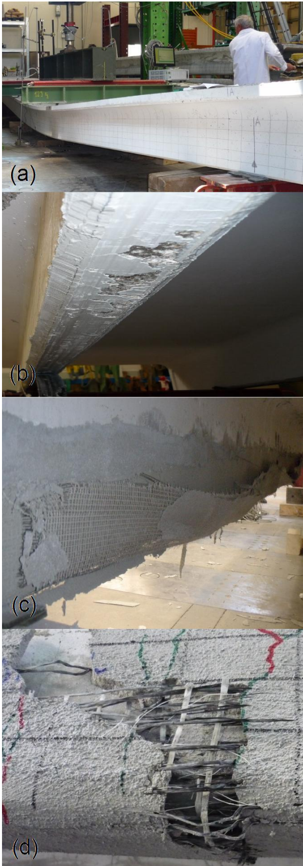
Figure 2: Failure of the beam TT00 (a), TTcl (b), TTsf (c), and TTcf (d).
