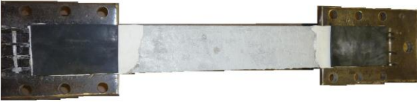
Figure 4: Setup of an FRCM carbon fibre specimen.
