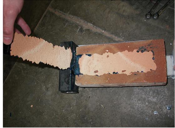
**Figure 5:** Typical failure observed for facing bricks
