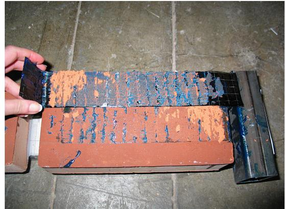
**Figure 6:** Typical failure observed for extruded bricks
