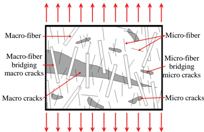
**Fig.1** Fiber bridging by hybridization of micro-fiber and macro-fiber (multi-level-reinforcement system) on crack surface
