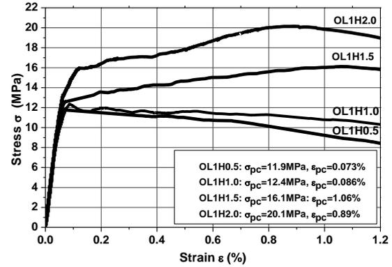
Fig.2 Tensile behavior of UHP-HFRCC developed in this study
