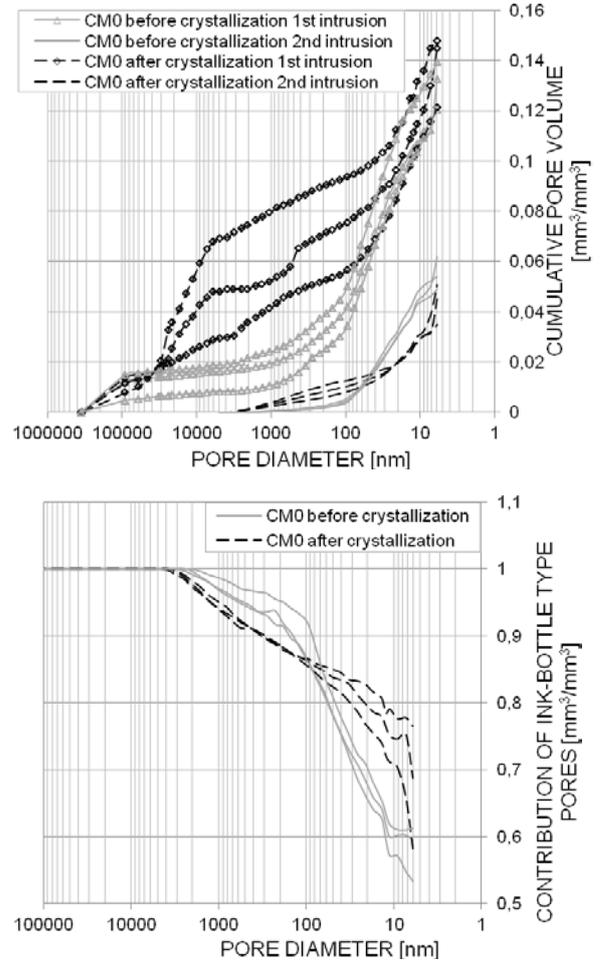
**Figure 1.** Comparison of a) cumulative pore volume and b) contribution of ink-bottle type pores obtained in MIP for CM0 samples before and after the crystallization test.
