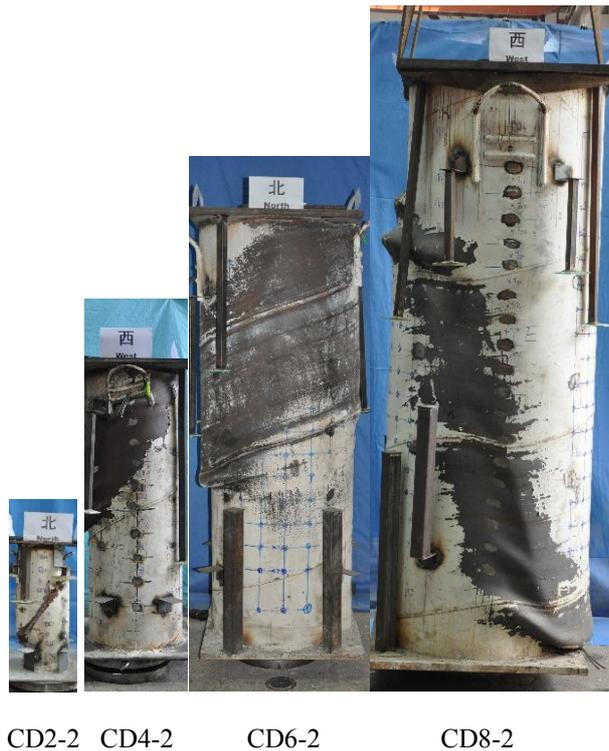
Figure 3: Final failure mode of the specimen.
