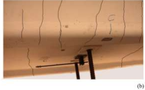
Figure 2: HPSFRC prestressed roof element: cross-section (a) and crack pattern (b) [2].
